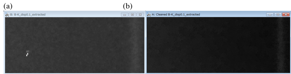
(a) An enlarged image of SR-EELS data of Boron K-edge. A spotty bright noise can be seen. (b) The enlarged image of the SR-EELS data at the same position as (a), but after the Filtering process. The noise is eliminated.
