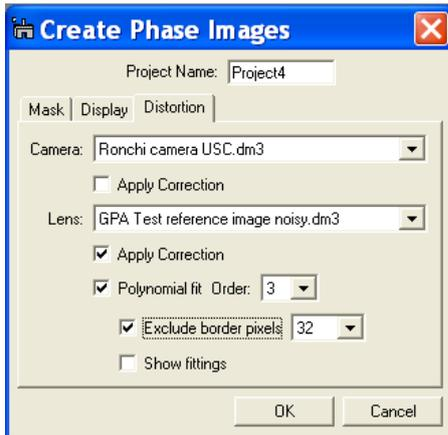
**Technical note:** projector lens distortions are theoretically a polynomial of order 3. It is therefore logical to use the same order for the fitting. However, higher orders can be used if necessary.
