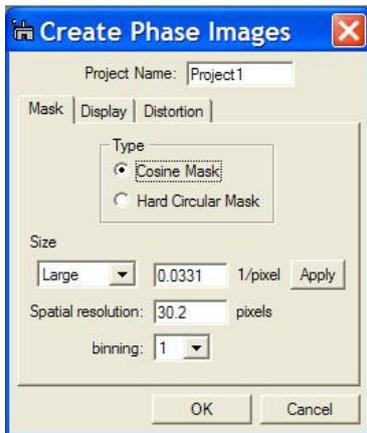
**Technical note:** the choice of the mask type (shape) is not that critical though the hard circular mask is to be avoided (only included for completeness). Hard masks in Fourier space introduce rippling effects in real-space, which is why smooth masks are preferred. Mask size is the most important parameter.
