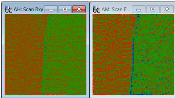
We can know see that the HAADF-STEM image was in fact taken of a twin boundary. There is neither expansion nor contraction in x and y, just a rigid-body rotation and shear of the crystalline lattice. Experiment yourself with the options to understand their effect.
