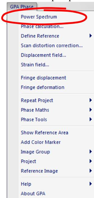
**Technical note:** in GPA, the image does not have to be a power of two in size (e.g. 512 by 512). However, streaks may appear in the power spectrum if greatly different in size from a power of two.
