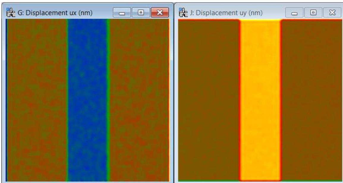
These two images represent the x and y-components of the 2D vector displacement,  $\mathbf{u}$ , respectively  $u_x$  and  $u_y$ . Since the original image was calibrated in nm/pixels, the displacements are automatically given in nm.
