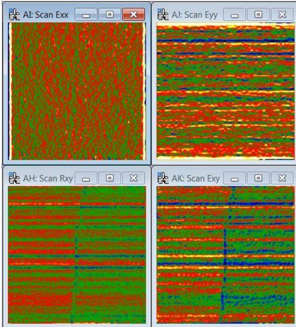
Notice that the vertical strain component,  $\epsilon_{yy}$ , the rotation  $\omega_{xy}$  and shear  $\epsilon_{xy}$  are all contaminated by horizontal streaks whereas the  $\epsilon_{xx}$  component is distortion free. The reason is that distortions come predominantly from the gradient of the phase images in the  $y$ -direction only.
