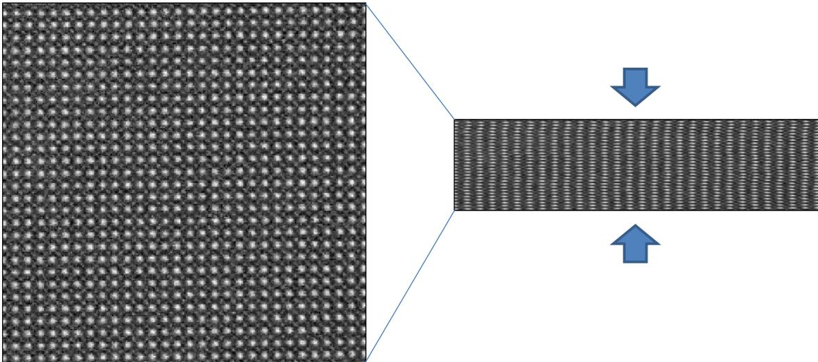
This is a well-known manifestation of the scan distortion. As the beam is scanned across the specimen from left to right it can jitter, due to interference from the electronics. At the end of a line it is swept back to start a new line. However, it does not arrive in exactly the correct place. The whole line can therefore have an additional displacement with respect to the previous line of scan: the so-called “fly-back” distortion. The result is highly visible in a phase image as shown below.
