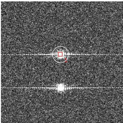
**Technical note:** the radius of the mask shows the area selected in Fourier space around the spot of interest. Decreasing the mask radius will produce smoother results but with less spatial resolution. The maximum recommended size is  $g/2$  corresponding to the large mask size.
