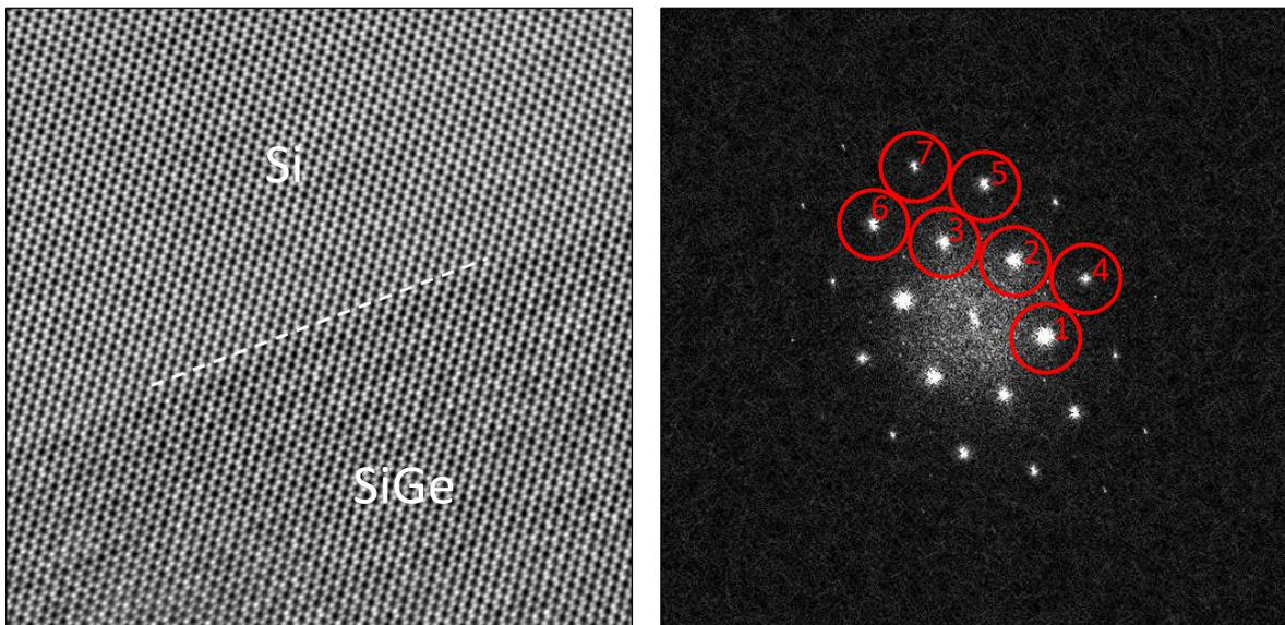
This image was taken on the aberration-corrected SACTEM microscope in Toulouse of SiGe grown epitaxially on a Si substrate [F. Houdellier & M.J. Hÿtch, *Microelectronic Engineering* 84 (2007) 460–463]. Select the 7 spots circled in the power spectrum with the **mouse tool** and calculate the amplitude and phase images. Use the **large mask size** and try and use the spots in the order indicated above. You should find the following images displayed after defining a reference area:
