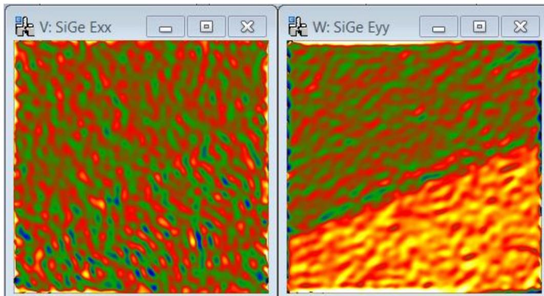
The improvement to the  $\varepsilon_{yy}$  component is impressive. What has been done? The information from all the phase images has been combined in a least-squares fitting routine to obtain the strain maps. In the default version, defined in the option menu, all the phase images are treated equally.
