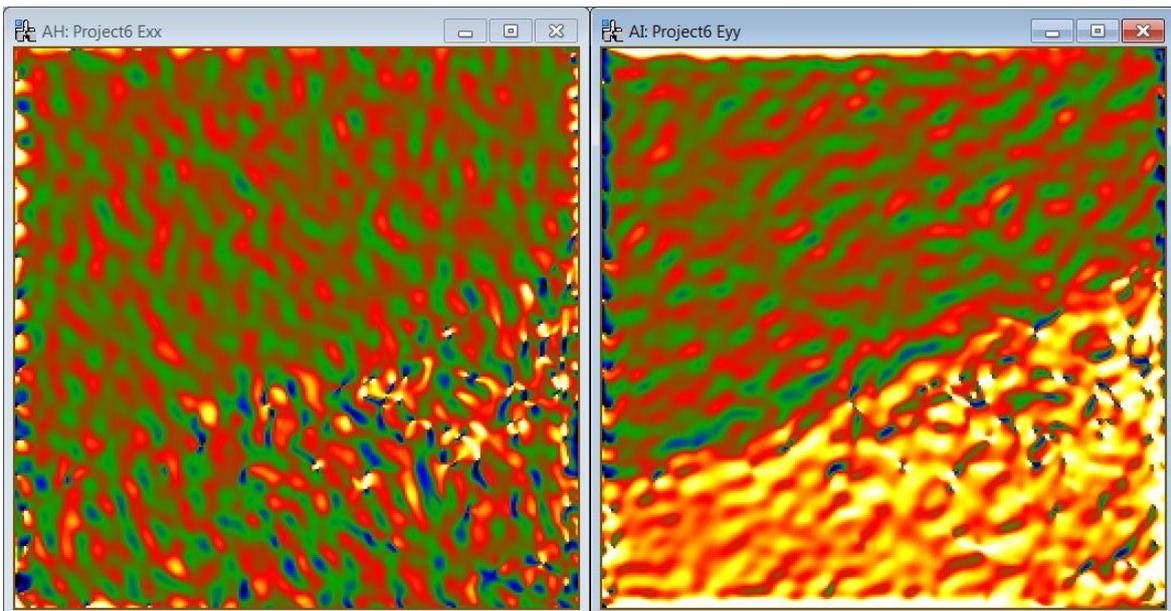
It can be seen that the strain maps are worse than with just 2 phase images! The reason can be found in the fifth phase image. The amplitude is almost zero in the SiGe layer for this set of fringes. Uncheck this phase image from the list and you will find a much better result.
