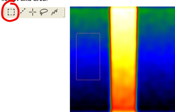
**Technical note:** choose an area of undistorted lattice as your reference area, recognised in the phase image as an area of uniform contrast or uniform gradient. For example, do not choose an area which straddles the interfaces. Having said that, please experiment.
