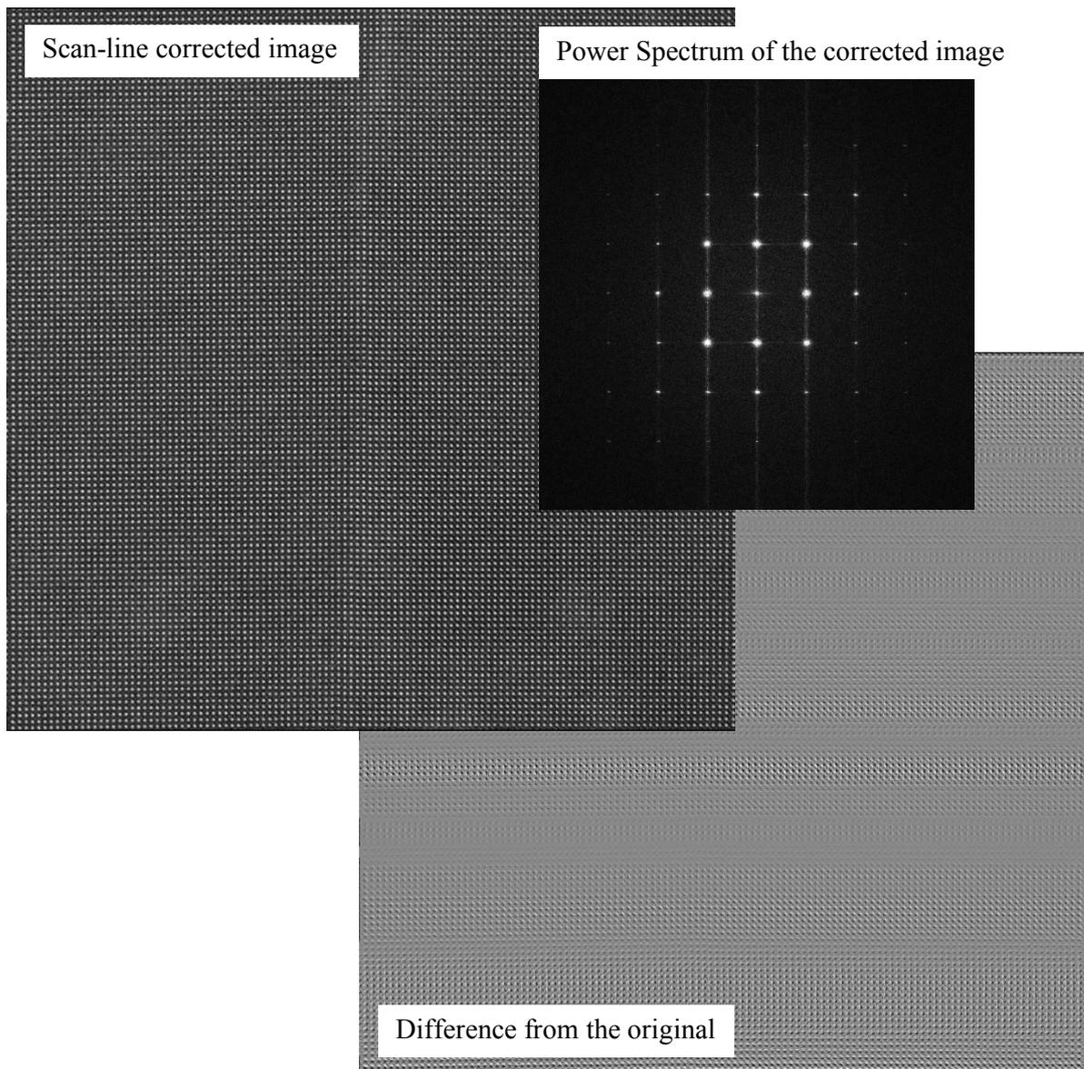
Scan-line distortion along the horizontal direction can be easily detected by eye, since the atomic lattice along the vertical direction looks wavy. Although it is difficult to detect the vertical distortion (namely, the variation of distance between the scan-lines), there should be a similar amount of distortion. The difference map above demonstrates that similar amounts of distortion appear along both directions, and the scan-line distortion can detect the distortions along both directions.
