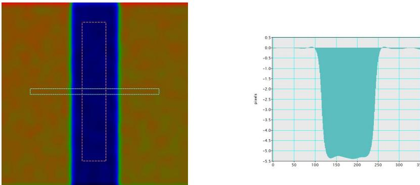
Since the original image is not calibrated (in nm/pixel) the displacement is given in pixels. Given the fringe spacing was 15 pixels, the exact displacement should be -5.252 pixels.
