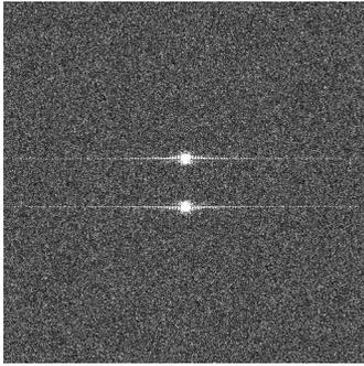
**Technical note:** the power spectrum is the modulus squared of the Fourier transform of the image. People are often surprised by the lack of a central spot in the power spectrum but this is normal for images where the mean intensity is zero, an important difference with diffraction patterns. The horizontal streaking of the spots is due to the interfaces in the image and is not, in this case, an artefact.
