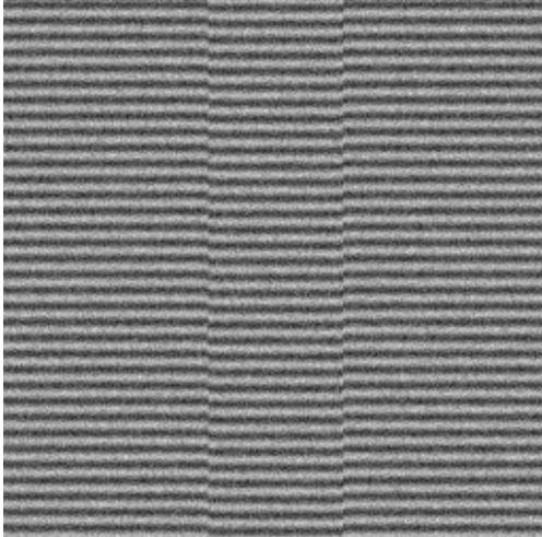
**Technical note:** you can find out how this image was created by looking at the script “GPA Test image 0.s” in the Phase Manual folder. Indeed, you can play with the image by changing the script, in particular the variable *dPhase* which determines the displacement.
