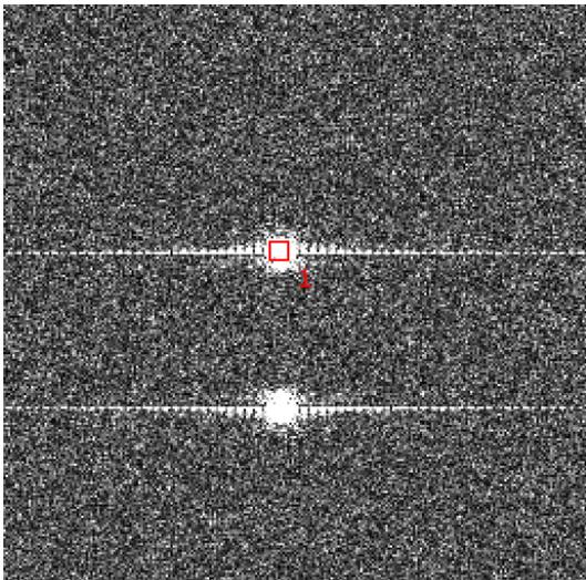
**Technical note:** do not worry about “hitting” the spot exactly. GPA will automatically hunt locally for the maximum intensity in the spot, even though the red square marks the actual pixel you hit.
