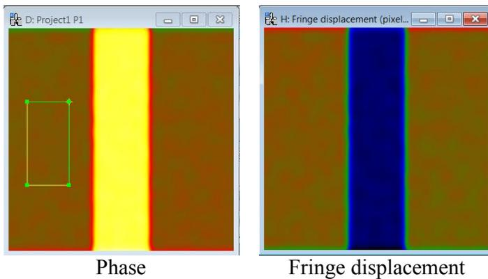
**Note:** the colour change between the phase and the displacement image is due to the negative sign in the phase-displacement equation. Look back to the original fringe image and you will see that the fringes are displaced in the negative g-direction (here, the g-direction is upward).
