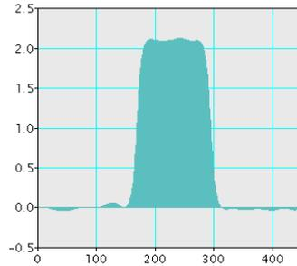
In the reference area the phase is zero and in the central band takes a value of 2.2 radians. This value can be verified in the original script used to create the image “GPA Test image 0”. Now choose the reference area in the central band, and you will see that the displacement is reversed. This illustrates the overall principle:
