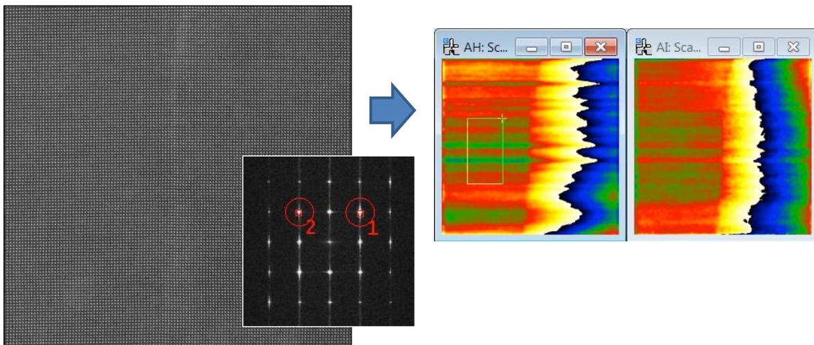
The phase images are not exactly what one would hope from a (almost) perfect crystal. However, we can see that the distortions form horizontal lines. The effect on the strain field is even more pronounced:
