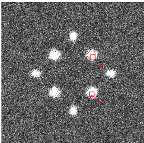
**Technical note:** in principle, it does not matter which two spots you choose, so long as their g-vectors are not parallel. In practice, the highest precision is obtained with low order spots and ones nearest to right-angles with respect to each other. Spots absent in the crystal structure are to be avoided (e.g. present due to double diffraction, misalignment etc.).
