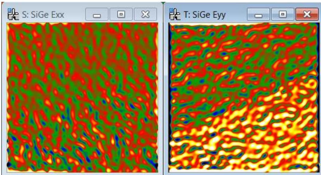
The  $\epsilon_{xx}$  component is on average zero, indicating that the interface is coherent between the SiGe and the Si. The  $\epsilon_{yy}$  component shows that the lattice parameter in the SiGe is larger than in the Si substrate. However, the image is rather noisy. Rather than reducing the **mask size**, let us see what using multiple phase images can do.
