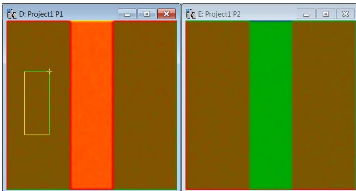
The phase images show that the central region is shifted with respect to the rest of the image. In this case, both phase image show a shift and therefore we need to combine the two phase images to determine the displacement vector (see Appendices for the equations). We can do this with the **Displacement field** command:
