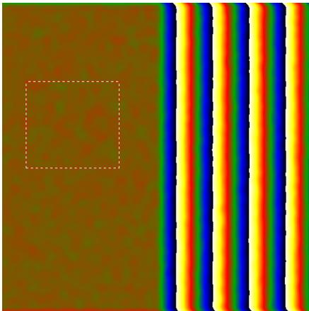
**Technical note:** do not worry about the “phase jumps” i.e. where the phase suddenly goes from black to white. This is quite normal and results from the normalisation of the phase between  $-\pi$  and  $\pi$ . Imagine the phase going round a circle moving seamlessly from 0 to  $\pi$  to  $-\pi$  and back again. No discontinuity is present in the underlying lattice images.
