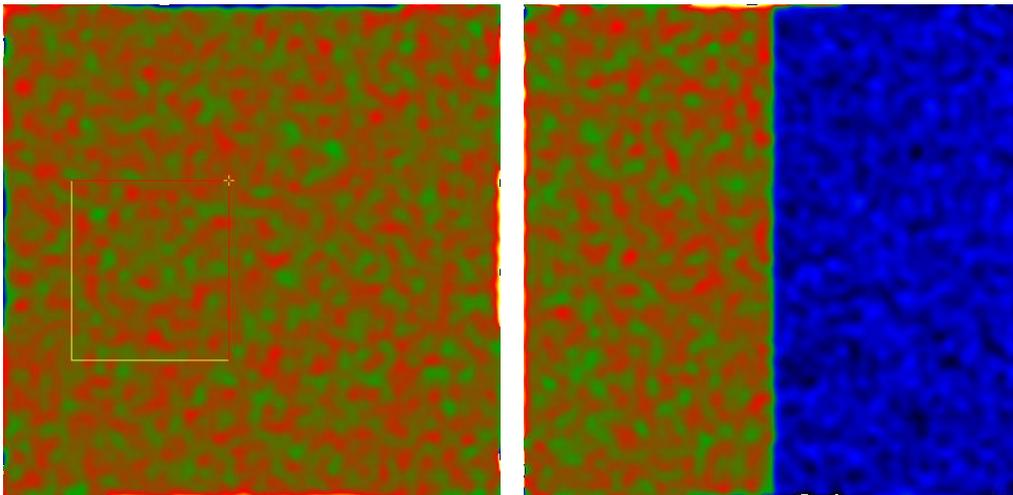
The results are much noisier than the previous example, because the noise in the reference image is effectively added to the image. To alleviate this problem, we have included in GPA Phase 3.0 the possibility of applying a polynomial fit to the reference image phases before subtracting them from the experimental phase. Recalculate the *GPA Test distortion* phases by ticking the **Polynomial fit** option:
